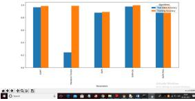
In above graph x-axis represents algorithm names and y-axis represents accuracy of train and test data and in all algorithms SVM with GA and SVM with PSO has got more accuracy compare to other algorithms.
